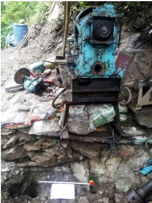
Figure 4-26: Core Drilling Being Operated in Re-Drilled Borehole HB – 1'
