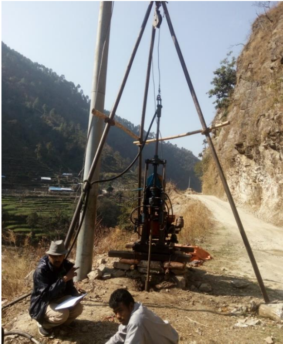
Figure 4-24: Core Drilling being Operated in borehole TT – 1
